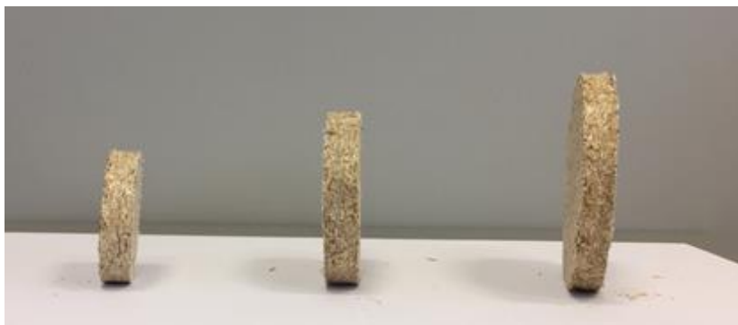
Fig.2 Crushed sunflower stalks briquettes of diameters 60, 80 and 100 mm
