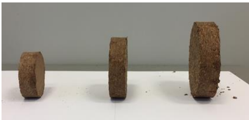
Fig.3 Crushed hazelnut husks briquettes of diameters 60, 80 and 100 mm
