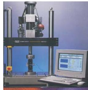
Dynamic and fatigue testing machine
