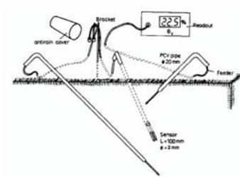
TDR probe field set up
