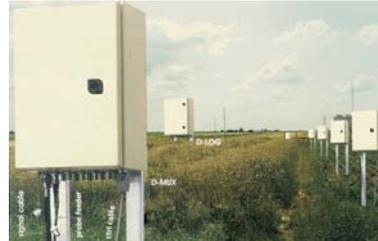
Field installation of TDR data logger
