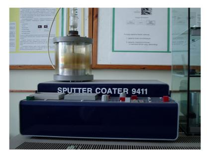
Fig. 2.33. Sputter coater with metallic coat thickness control (Au, Pt).
