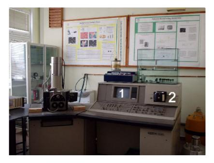
Fig. 2.29. A scanning electron microscope (TESLA BS 340). Control monitor /1/. Monitor-camera unit /2/.
