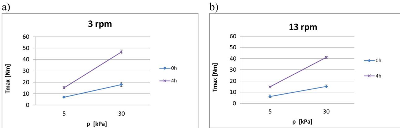
Fig. 5. Maximum values of torque  $T_{\max}$  as dependent on normal pressure and compression times of 0 and 4 h for two rotational speeds 3 rpm (a) and 13 rpm (b).
