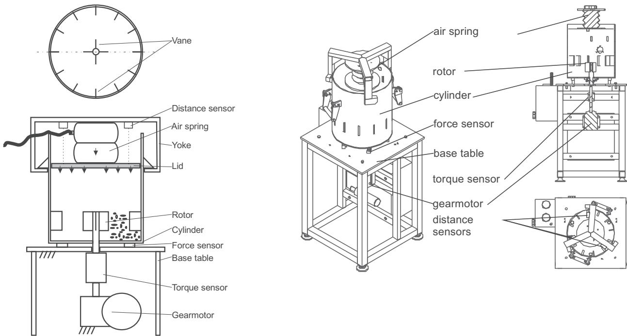
**Fig. 1.** The biomass vane shear tester VST.
