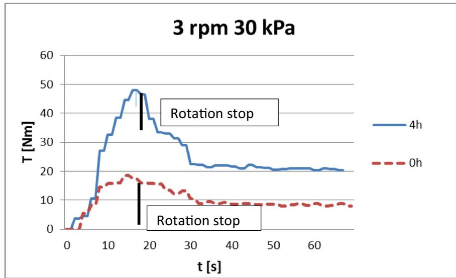
Fig. 4. Torque vs. time curves obtained at normal pressure of 30 kPa, for rotational speed of 3 rpm, after compressed for 0 h and 4 h.
