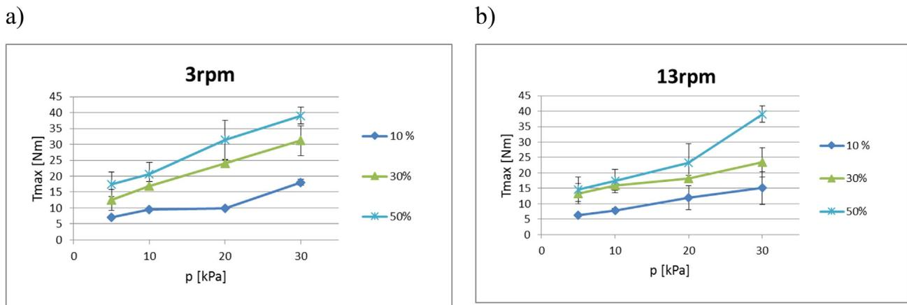
**Fig. 6.** The evolution of the maximum torque with normal pressure for material with different moisture contents, at rotational speeds of: (a) 3 rpm and (b) 13 rpm.
