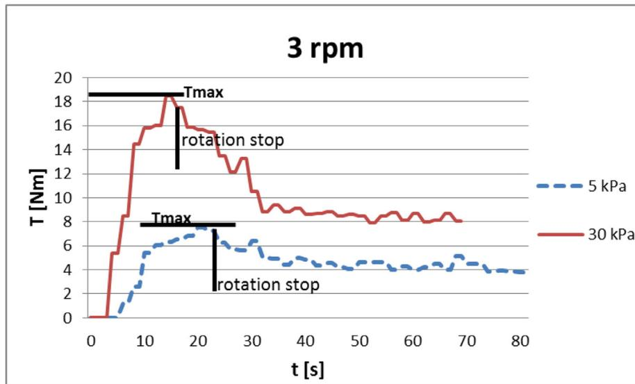
Fig. 2. Examples of torque-time curves obtained at normal pressure of 5 kPa and 30 kPa for rotational speed of 3 rpm.
