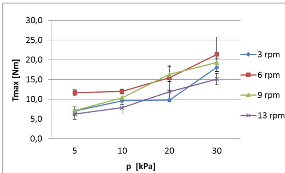
Fig. 3. Characteristics of maximum torque vs. normal pressure  $T_{max}(p)$  for four values of rotation speed.
