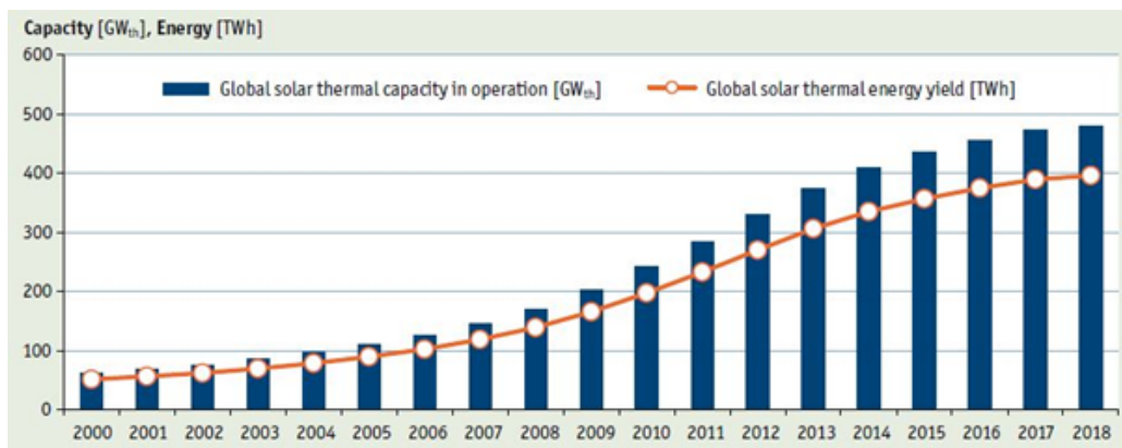
Fig. 1 Global solar thermal capacity and energy yield for the period of 2000-2018
