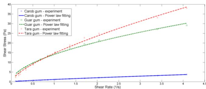
Fig. 1. Effect of shear strain rate on the shear stress
