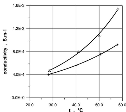
Fig. 2. Temperature dependence of maize conductivity for rape oil seeds Belinda at the moisture content of 20.2 % ( $\Delta$ ) and at 19.5 % (+)
