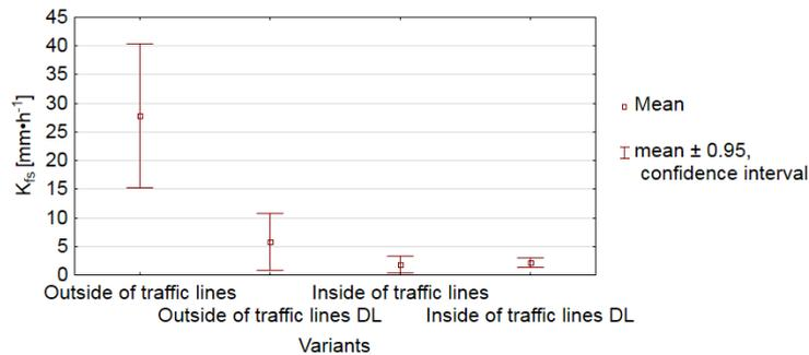
Fig. 1. Soil infiltration parameters across the variants (DL – deep loosening)
