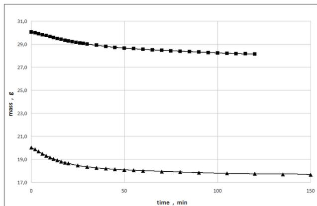
Fig. 1. Time dependence of the mass of samples, (CTF-8C) grains ( $\square$ ) and wheat (Magister) ( $\Delta$ )
