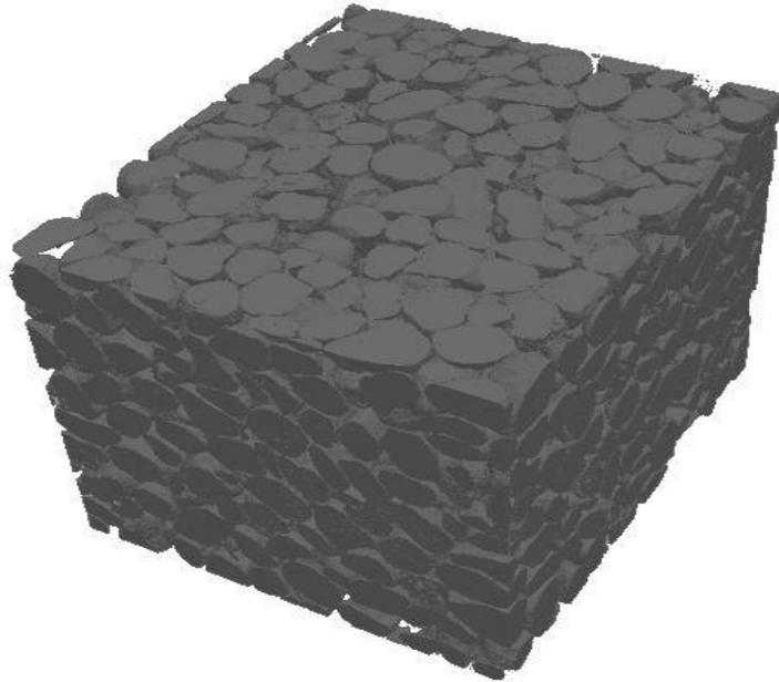
Fig. 1: An example of 3D-reconstruction of the soil sample.
