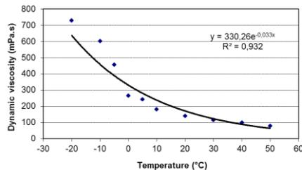
Fig. 1. Dynamic viscosity for Plantohyd 46S Fig. 2: Dynamic viscosity for Plantohyd 40N
