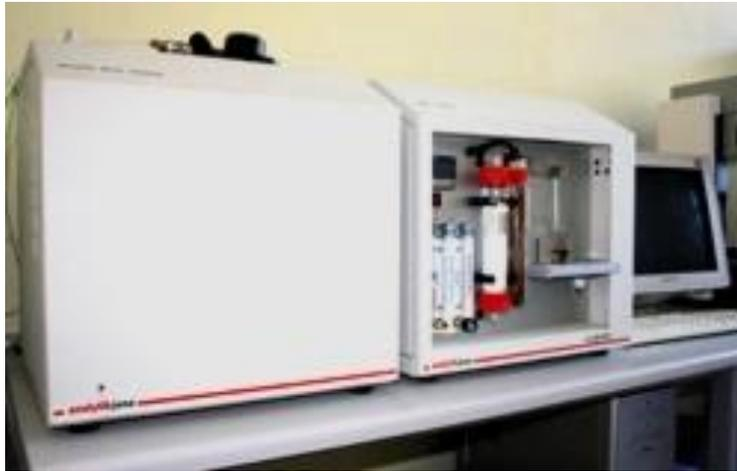
Fig. 2. Carbon and Nitrogen Analyzer TOC Multi N/C 2000, HT 1300 Analytik Jena
