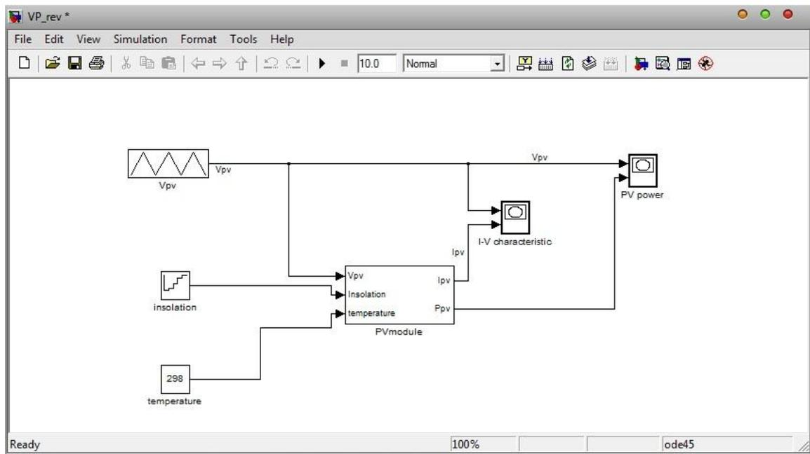
Fig. 1. A diagram block for single diode model of PV system
