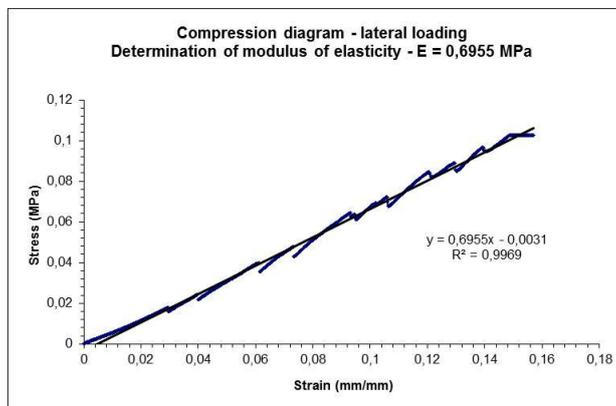
Fig. 1 Compression stress – strain curve of apple fruit Golden Delicious in the lateral loading
