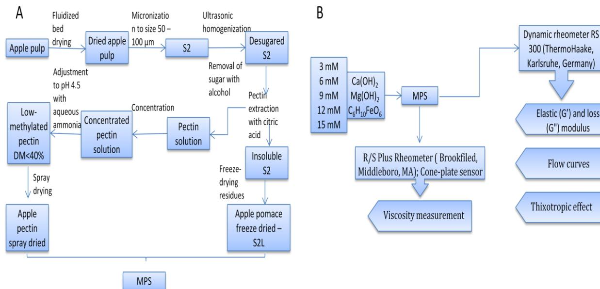
Fig. 1. Production flowchart (A) and scheme of rheological properties' determination of cell wall polysaccharide matrix (MPS) (B).
