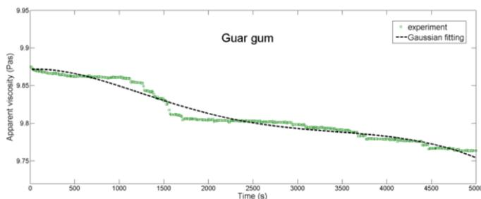
Fig. 3. Time dependence of the apparent viscosity – guar gum solution
