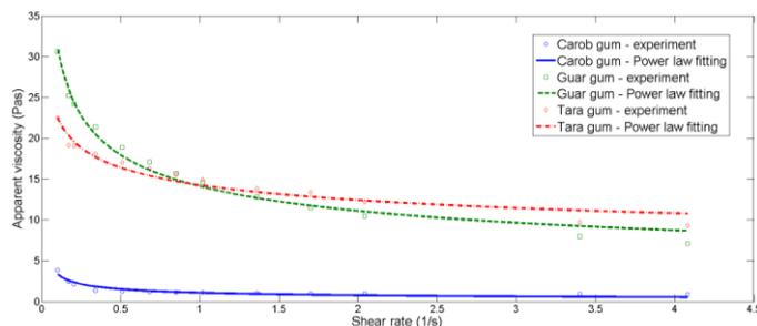
Fig. 2. Viscosity of the hydrogels
