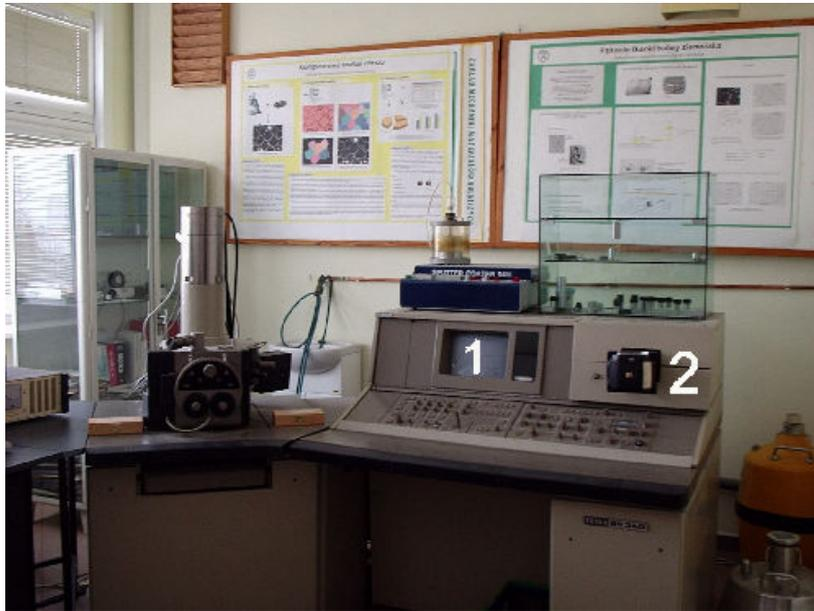
**Fig. 2.29.** A scanning electron microscope (TESLA BS 340). Control monitor /1/. Monitor-camera unit /2/.
