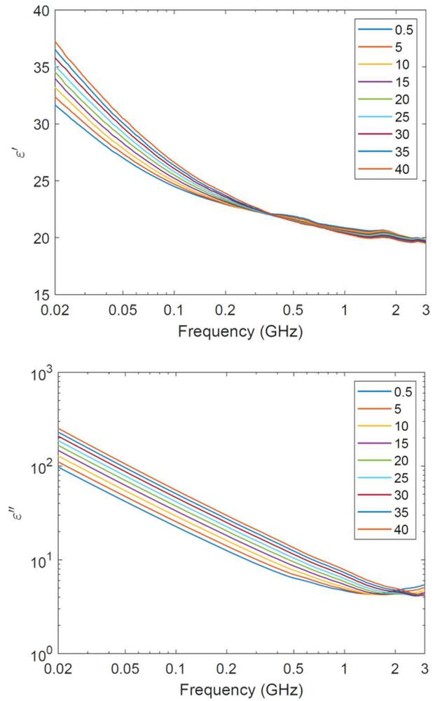
Fig. 2. Real (top) and imaginary (bottom) parts of complex dielectric permittivity of soil of 38% moisture content at various temperatures given in the legend in °C.
