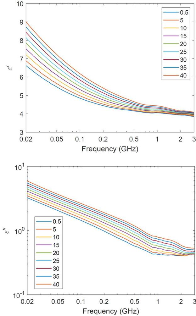
Fig. 1. Real (top) and imaginary (bottom) parts of complex dielectric permittivity of soil of 9% moisture content at various temperatures given in the legend in °C.
