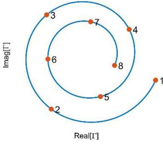
Fig. 2. Reflection coefficients of the antenna measured by an ideal six-port-based CW radar for eight target's positions equally distributed over the distance equal to wavelength.
