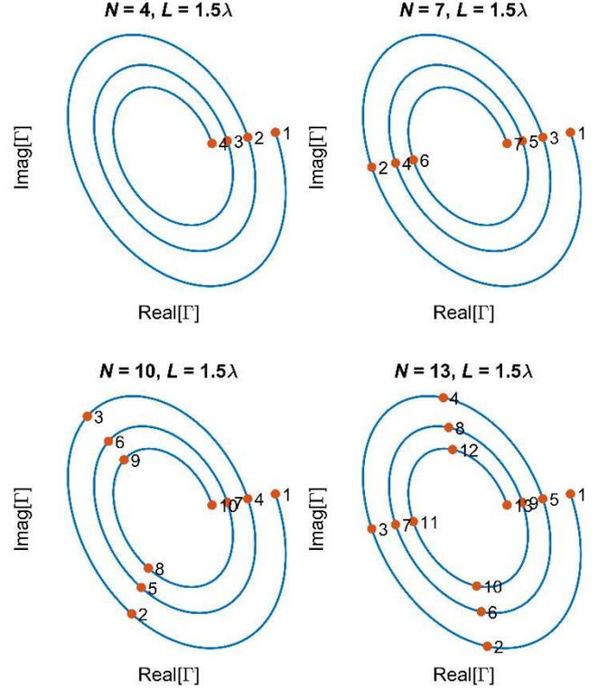
Fig. 3. Reflection coefficients of the antenna measured a real uncalibrated six-port-based CW radar for different number of target's positions  $N$  and fixed spread  $L = 1.5\lambda$  defined as a distance between the first and the last position.
