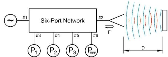
Fig. 1. A generic diagram of a six-port-based CW radar.
