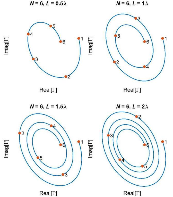
Fig. 4. Reflection coefficients of the antenna measured a real uncalibrated six-port-based CW radar for fixed number of target's positions  $N = 6$  and different spread  $L$  defined as a distance between the first and the last position.
