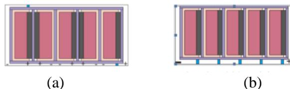
Fig.1. Schematic configuration of monolithic DSSC module with (a) series, and (b) parallel interconnection.
