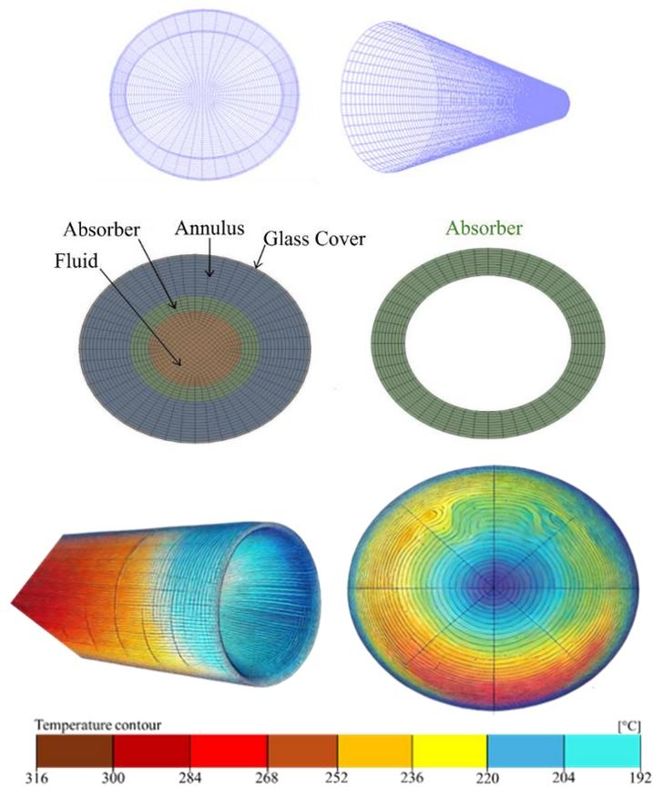
Fig. 1. Computational modelling and heat distribution of CPC absorber
