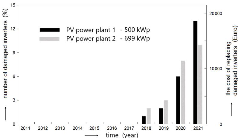
Fig. 2. The number of damaged inverters in the case of two selected PV power plants.
