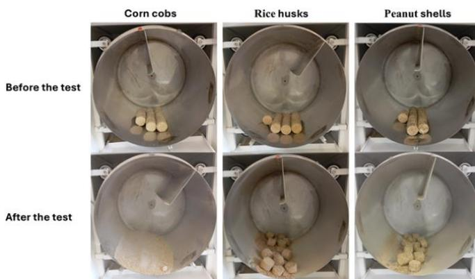
Fig. 1. Mechanical durability test.
