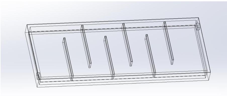
Fig. 1. Schematic diagram of a solar air collector
