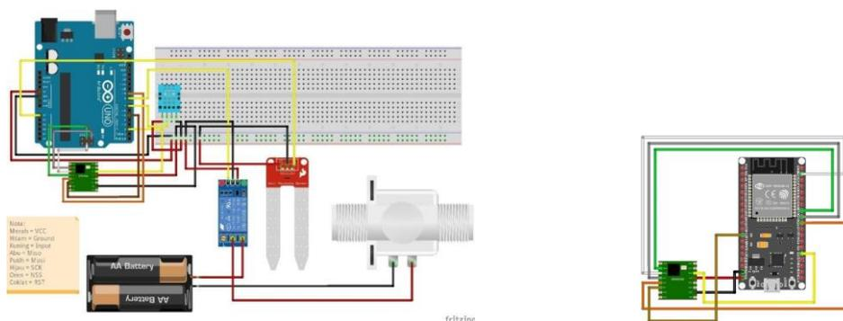
Fig. 1. Wiring Diagram on Transmitter (Left) and Receiver (Right) side.
