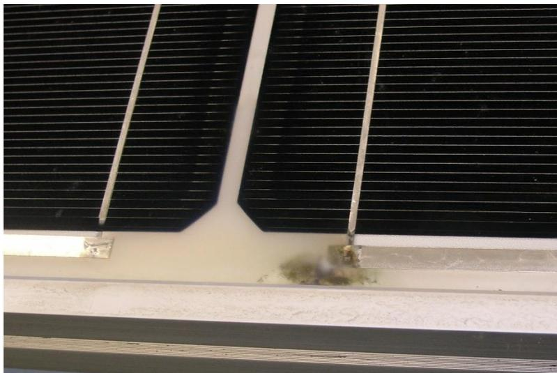
Fig. 1. The conductive channel between the electrode and the grounded frame of the PV panel.
