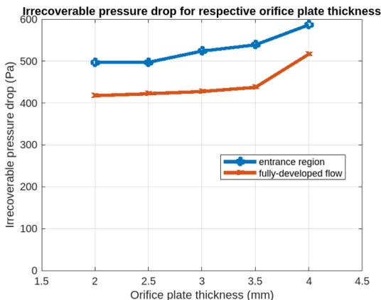
Fig 1. Simulation results of pressure drop in respective orifice plate thickness for both entrance region and full-developed flow region
