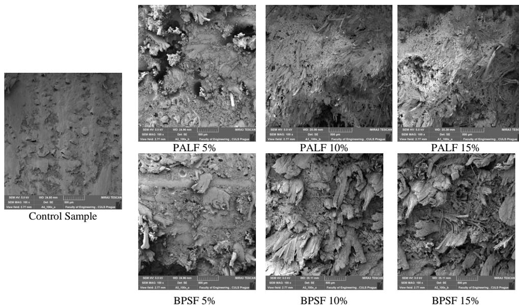
Fig.2. PALF & BPSF Composite Scanning Electron Microscopy (SEM)
