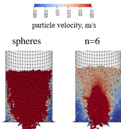
Fig. 2. Profiles of particle vertical velocities for spheres and hexahedrons.
