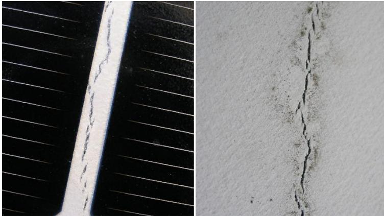
Fig. 1. Degradation of the polymer on the back side.
