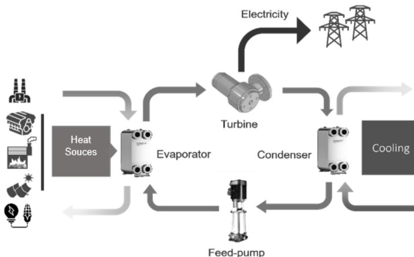
Fig. 1. Schematic layout of basic ORC with various heat sources, adapted from (Source: ecoprius.pl)
