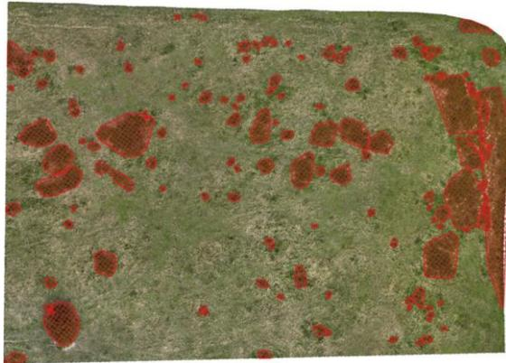
Fig. 1. Example illustration of RGB thresholding applied to pasture orthophoto to identify potential weed clusters (red areas).
