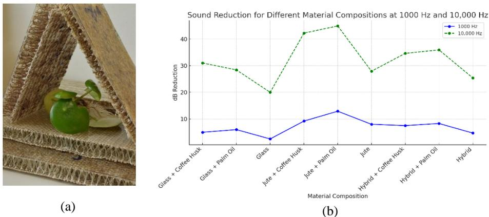
**Figure 1.** (a) An image of the (3DJGF); (b) Bar illustrating the sound reduction levels for different materials at both 1000 Hz and 10,000 Hz.
