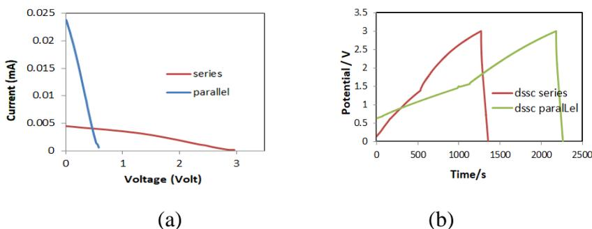
Fig. 2. Comparison between (a) current-voltage (I-V) curves and (b) photo-charging profiles for monolithic DSSC module with series and parallel interconnection.
