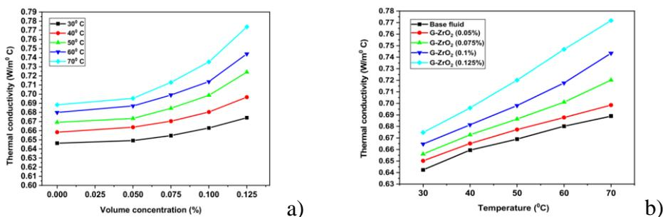
Fig. 1. Thermal conductivity of nanofluid:
