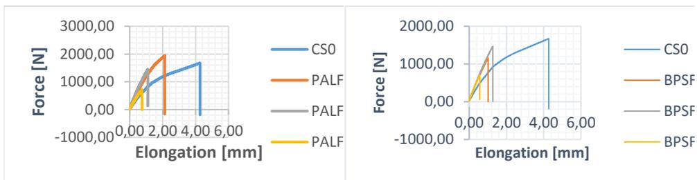
Fig.1. Load Force vs. Elongation of PALF & BPSF Composite
