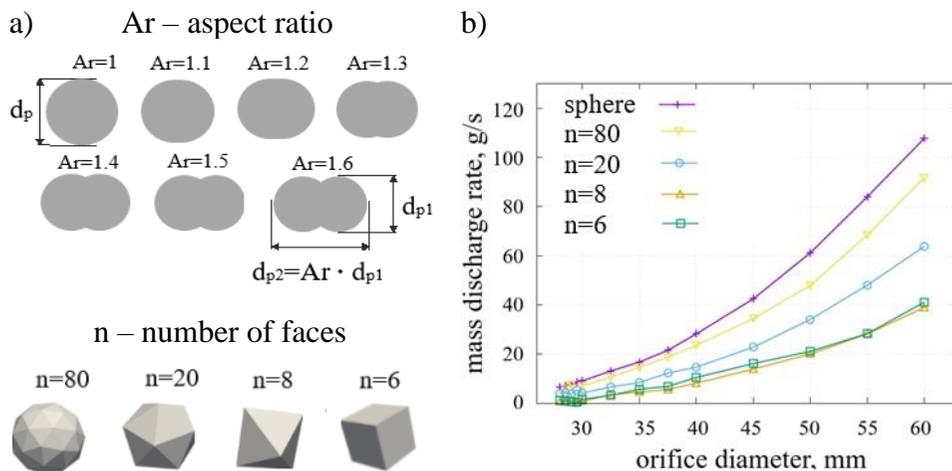
Fig. 1. Particles used for DEM simulations (a) and mass discharge rates for various orifice size and particle shape (b).
