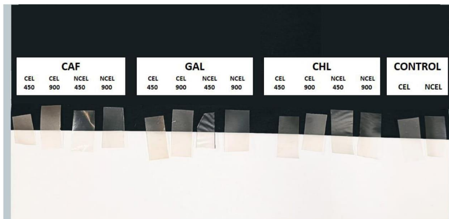
SM Fig. 1. Photo of composites with selected phenolic acids gallic acid (GAL), chlorogenic acid (CHL), and caffeic acid (CAF) adsorbed on the surface at a concentration of 900 ppm and 450 ppm on cellulose (CEL) and nanocellulose (NCEL) based.
